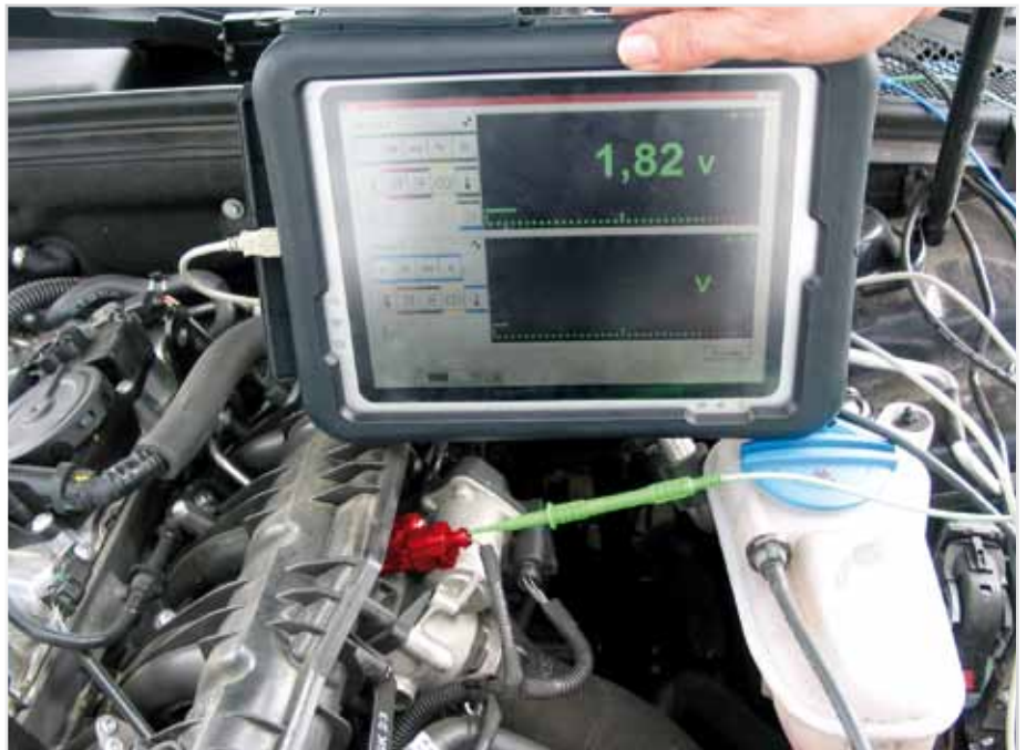
Measurement of output voltage on intake manifold pressure sensor (highlighted) in Audi A4 TFSI
